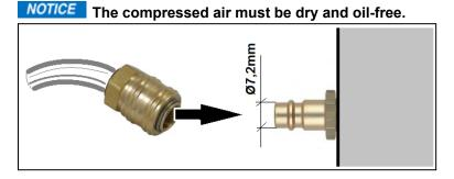
• The operating pressure of the compressed air supply must be a minimum of 3 bars and maximum of 4 bars.
